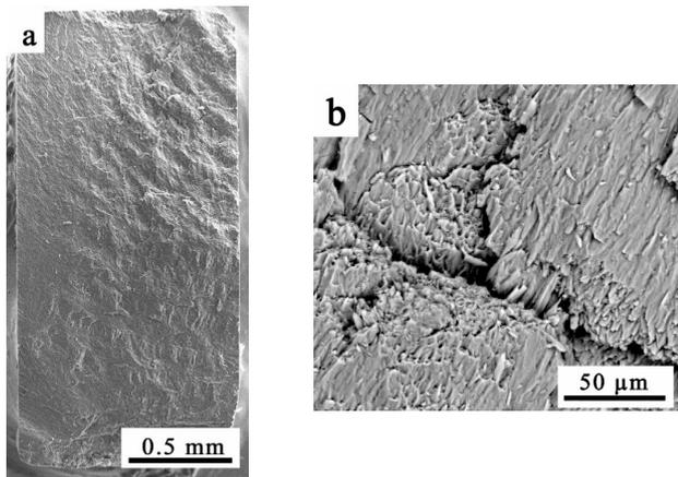
**Fig. 4.** Fracture surface (SEM) of human tooth enamel under Brazilian testing (diametral compression) in liquid nitrogen (77 K): a – low magnification; b – high magnification.
