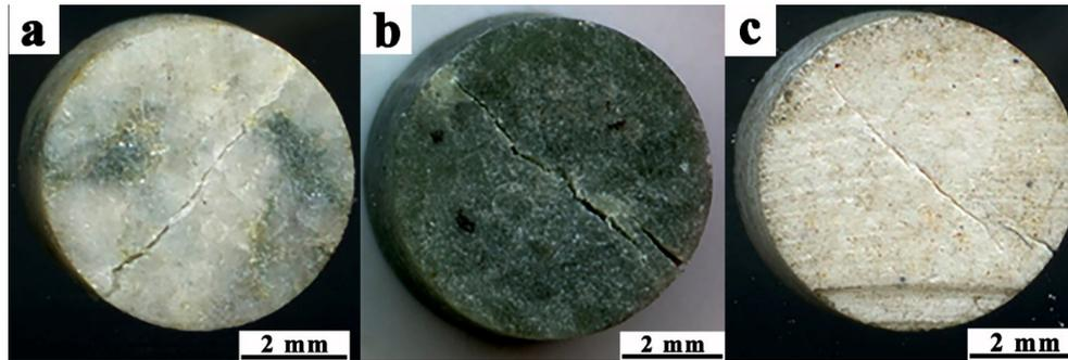
**Fig. 8.** Cracks on the working surface of some rock materials under diametral compression (Brazilian testing) in air at 300 K (optical microscope): a – granite; b – serpentine; c – plasma-sprayed  $\text{Al}_2\text{O}_3$ .
