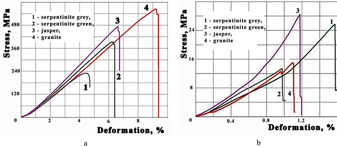
Fig. 2. Deformation curves of some rocks in air at 300 K: a – under uniaxial compression; b – under Brazilian testing (diametral compression).
