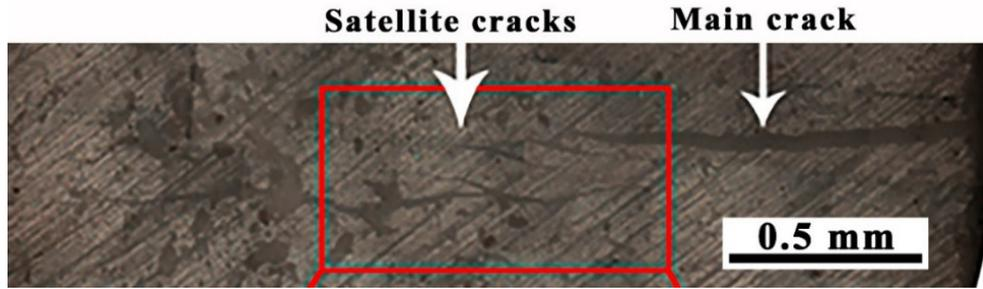
**Fig. 7.** Main crack with satellite cracks ahead on the working surface of human tooth enamel under Brazilian testing (diametral compression) in air at 300 K (light microscope).
