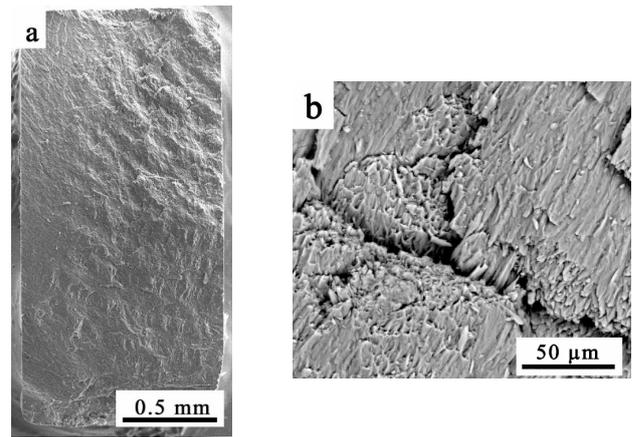
**Fig. 5.** Fracture surface (SEM) of human tooth enamel under Brazilian testing (diametral compression) in air at 300 K: a – low magnification; b – high magnification.
