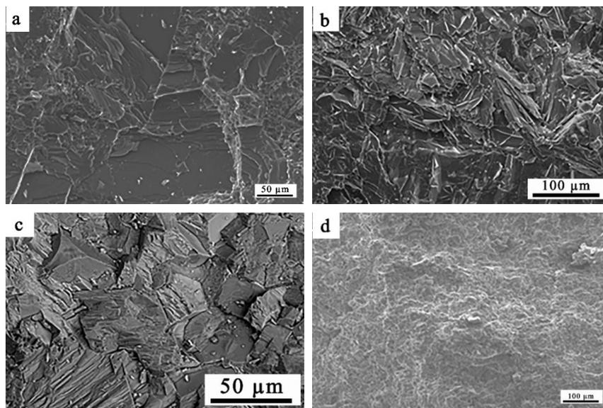
**Fig. 6.** Fracture surface (SEM) of some rocks under Brazilian testing (diametral compression) in air at 300 K: a – granite; b – serpentine; c – jasper; d – plasma-sprayed  $\text{Al}_2\text{O}_3$ .
