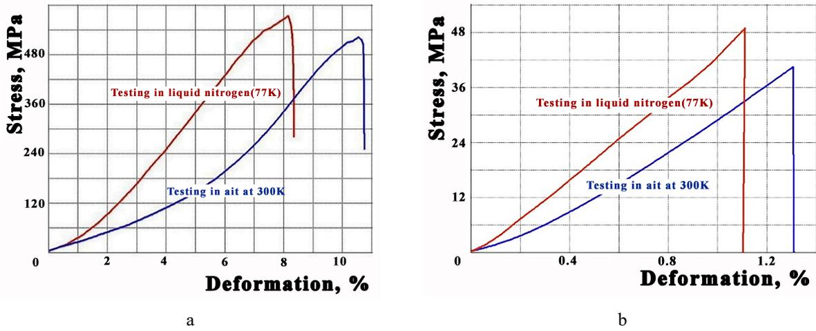
Fig. 1. Deformation curves of human tooth enamel in air at 300 K and in liquid nitrogen (77 K): a – under uniaxial compression; b – under Brazilian testing (diametral compression).
