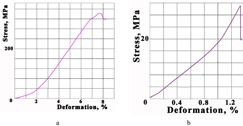
Fig. 3. Deformation curves of plasma sprayed Al<sub>2</sub>O<sub>3</sub> in air at 300 K: a – under uniaxial compression; b – under Brazilian testing (diametral compression).
